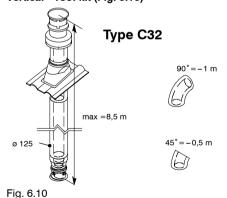
This kit allows vertical termination of the flue pipe through the roof. The kit is 1.2 m in length. Extension pieces (Co-axial) are also available which allows the flue system to be extended to a total overall maximum permissible length.
